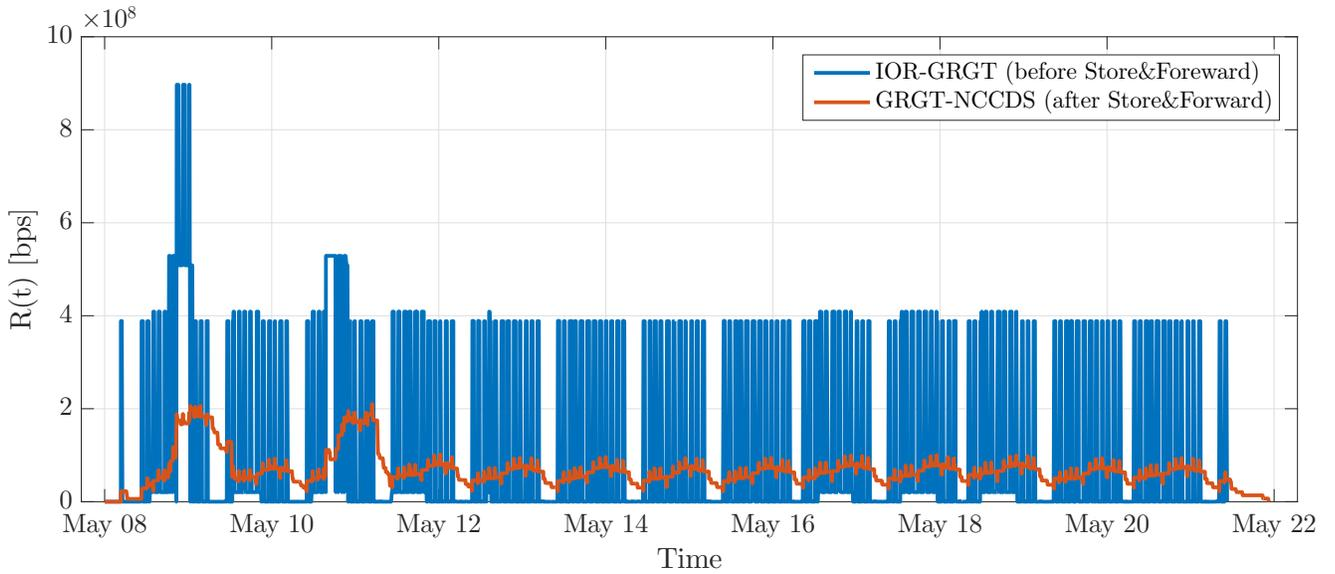
Figure 8: Smoothing Effect of Store and Forward at GRGT node
