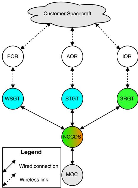
Figure 6: Current SN Architecture
